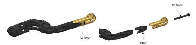
Unscrew M4 screw on the tip of the lever.
